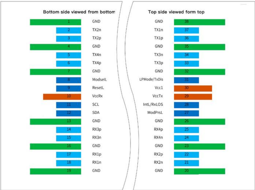
Figure 2 QSFP112 Module Contact Assignment
