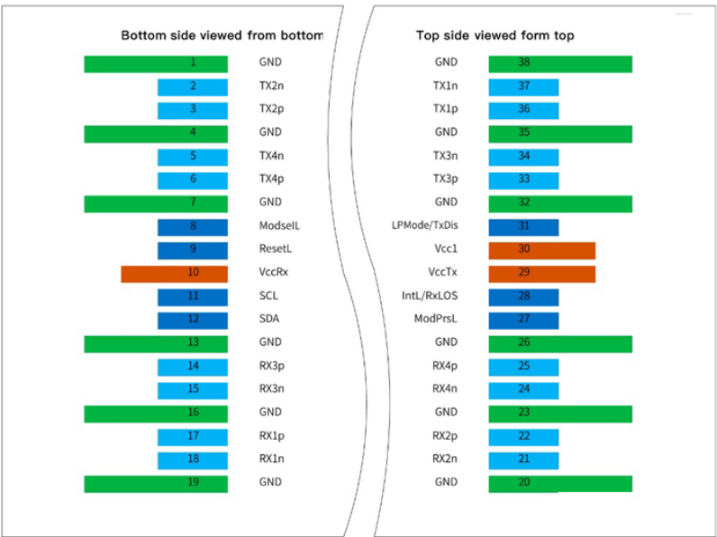
Figure 2 QSFP112 Module Contact Assignment
