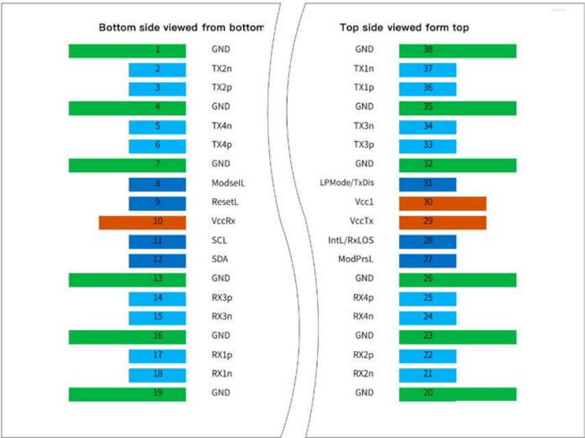
Figure 2 QSFP112 Module Contact Assignment
