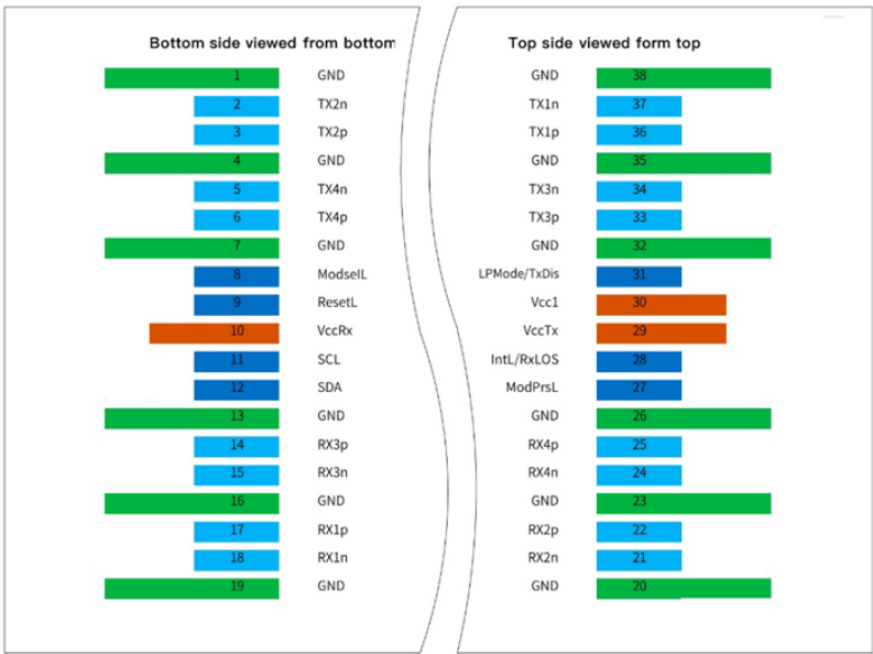
Figure 2 QSFP112 Module Contact Assignment
