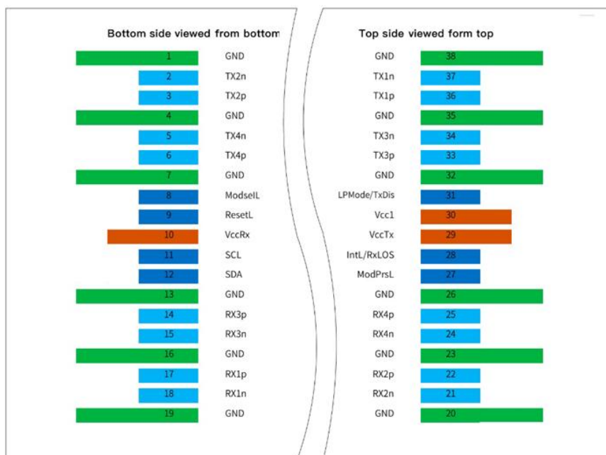
Figure 2 QSFP112 Module Contact Assignment
