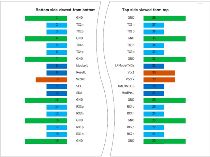
Figure 2 QSFP112 Module Contact Assignment
