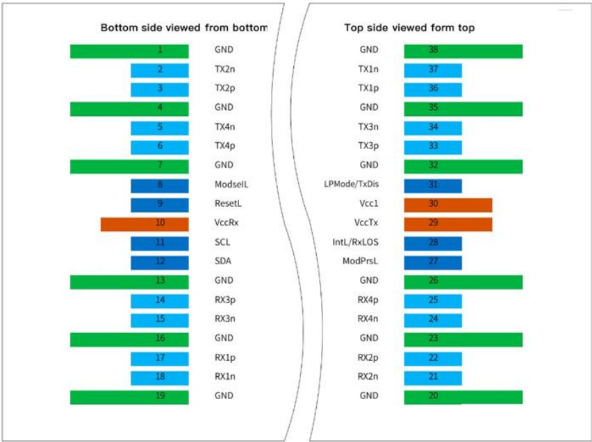
Figure 2 QSFP112 Module Contact Assignment
