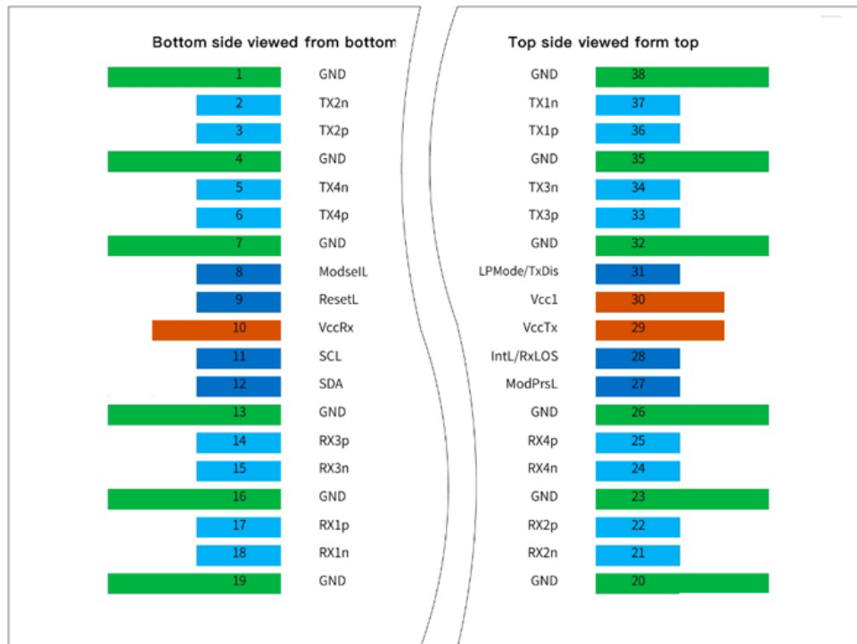
Figure 2 QSFP112 Module Contact Assignment
