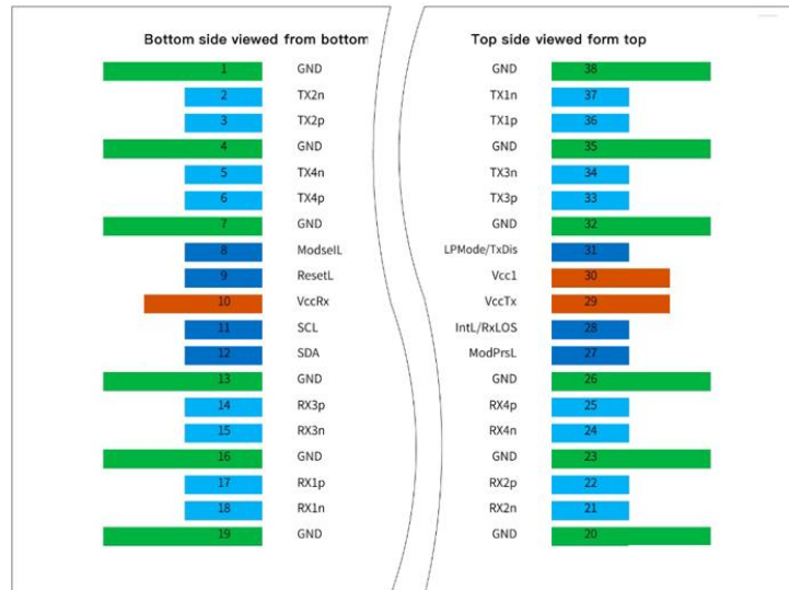
Figure 2 QSFP112 Module Contact Assignment
