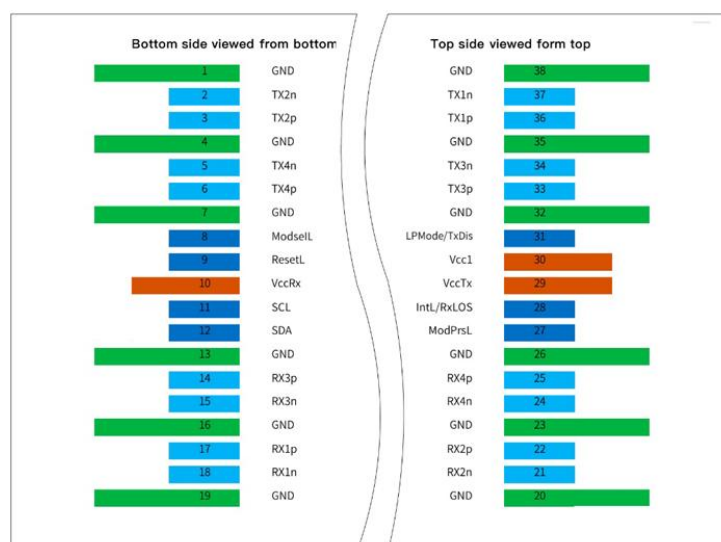
Figure 1 QSFP112 Module Contact Assignment
