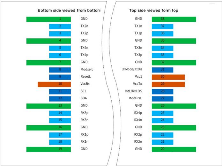
Figure 1 QSFP112 Module Contact Assignment
