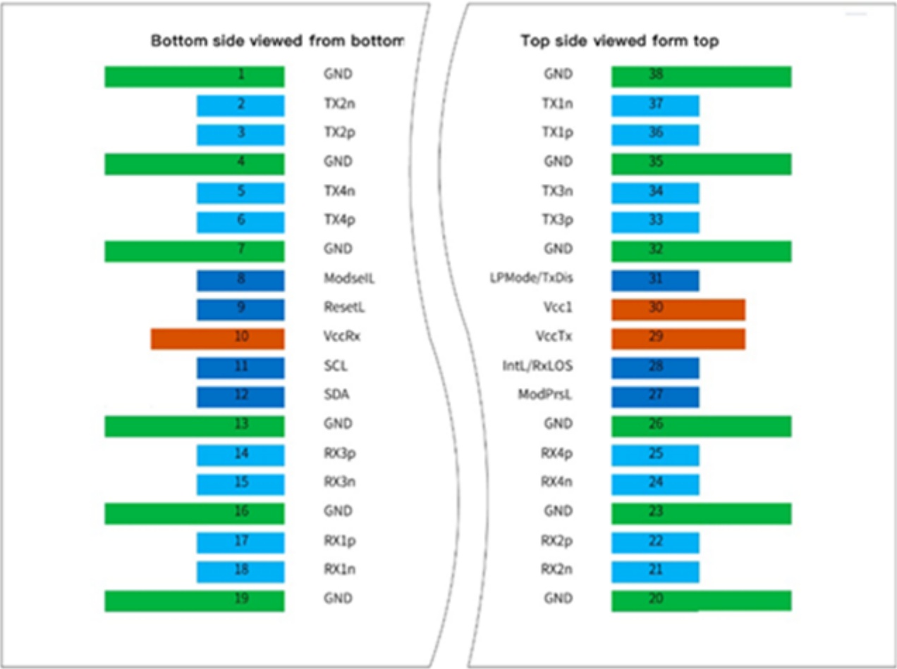
Figure 1 QSFP112 Module Contact Assignment
